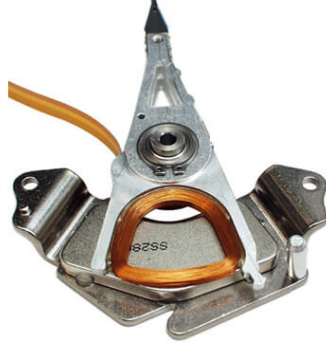
Figure 5.1: A VCA used in disk drives. Image taken from SDM Magnetics [47]
